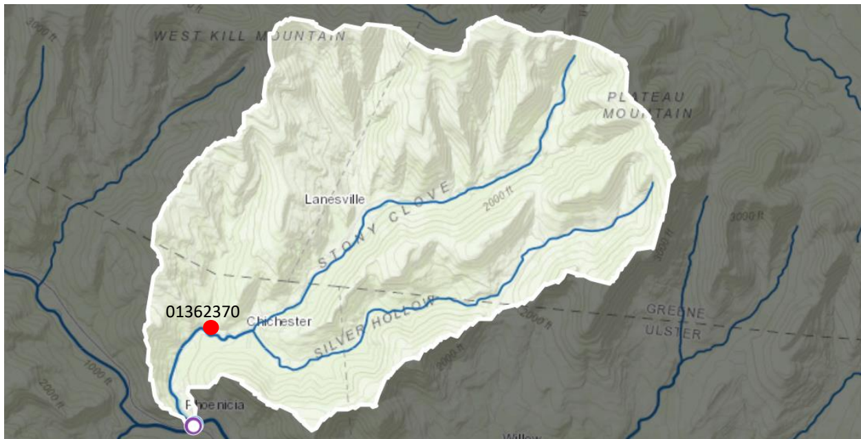
Figure 14. Watershed delineation from the headwaters of the drainage basin for Stony Clove Creek. The red dot is site number 01362370 (Stony Clove Creek at Chichester, NY). A plausible area of the watershed that could be contributing to turbidity during the first stage of the streamflow-independent event at Stony Clove Creek in 2015 is shown in blue (only the stream is highlighted, as the main source of turbidity at this stage is most likely from in-stream suspension). The second main stage of the event is the peak turbidity, where the potential source contributions to turbidity are from the influx of sediment from the mass wasting event and in-stream scouring. Hypothetical source contributions to turbidity near site 01362370 from land surface erosion at this stage can come from anywhere upstream. The source could be confirmed by comparing upstream and downstream gauges to one another for their respective turbidity values.
