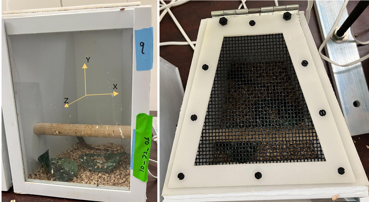
Fig. 4: Cage used to house lizards for the stimulus experiments. The lines indicate arbitrary axes assigned by me to help describe the physical nature of the cage. The cage was 19x19x24 cm. Each cage had the same organization of a rocky substrate, faux leaf, and a perch. Each cage also had its own heating lamp above the y-axis (not pictured).
