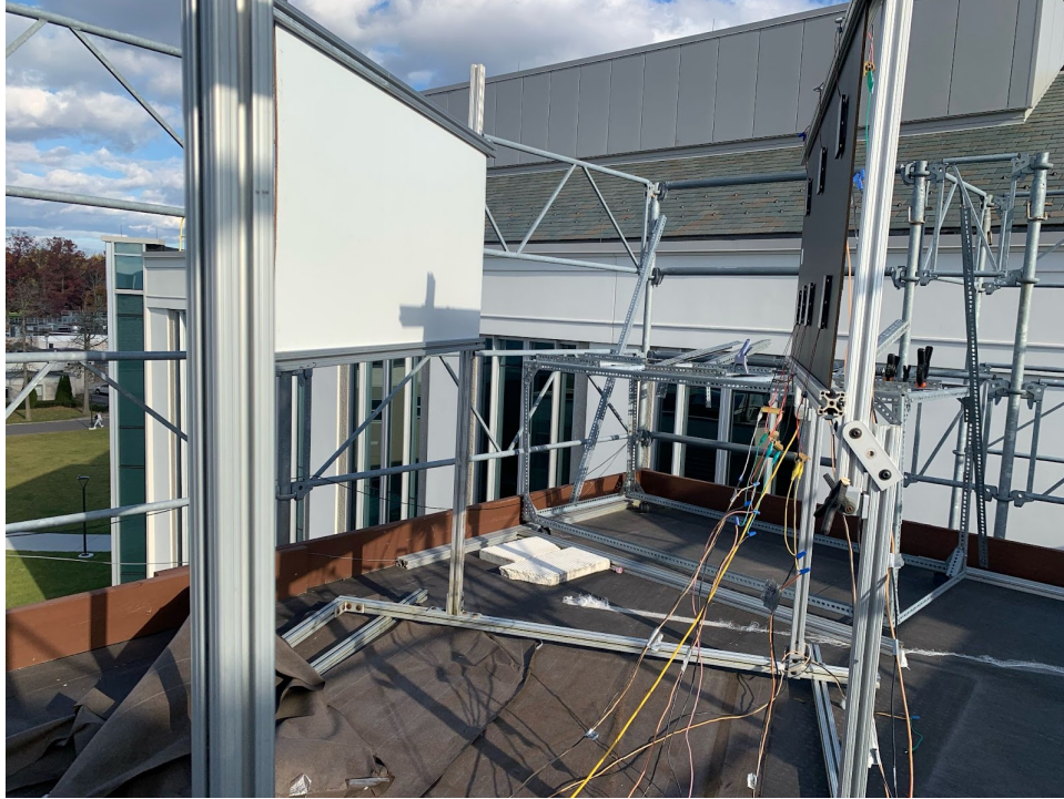
Figure 10: Reflector-collector set-up with a separation distance of 1m.
