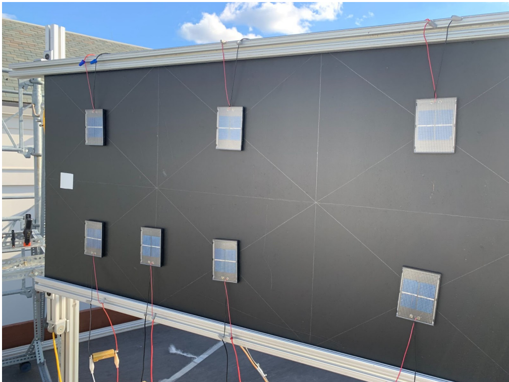
Figure 9: Set-up of cells on the collector.
