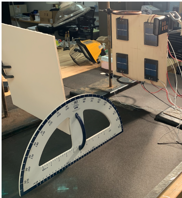
Figure 13: Indoor bifacial PV reflector-tilt set-up.
