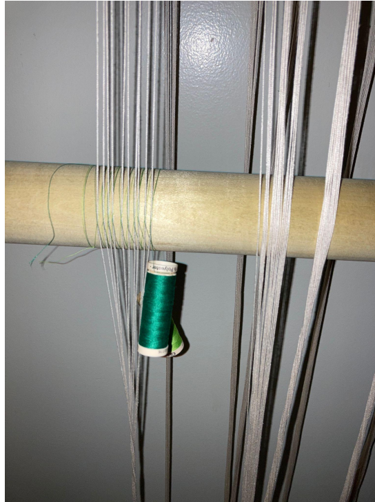
Figure 10: Threads Attached to Shed Bar
