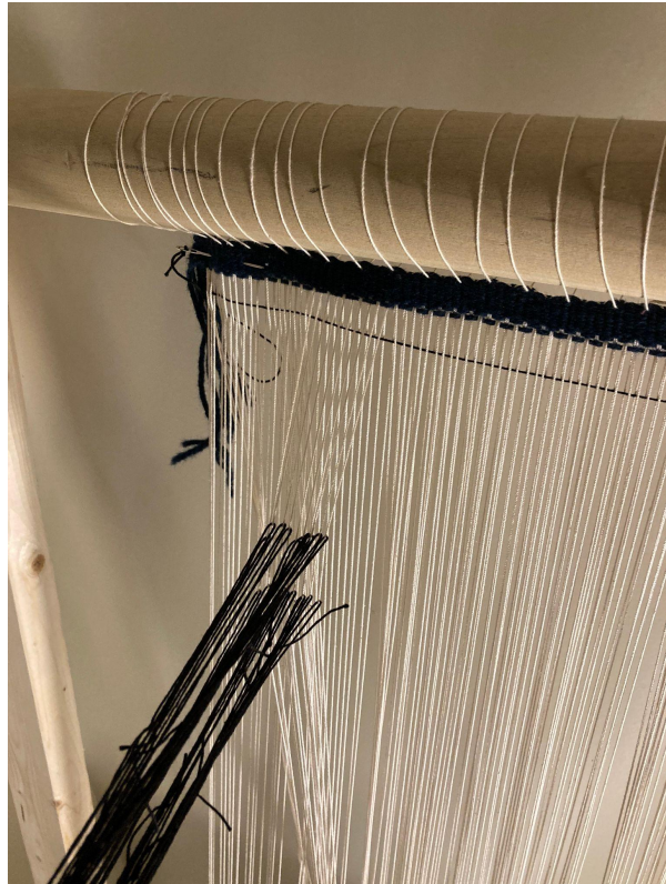
Figure 11: Threads Attached to Heddle Rod
