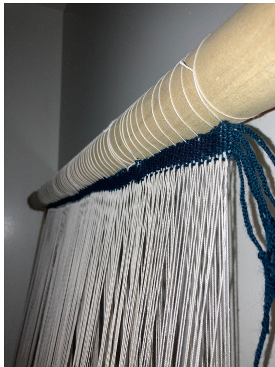
Figure 9: Heading Band Attached to the Loom
