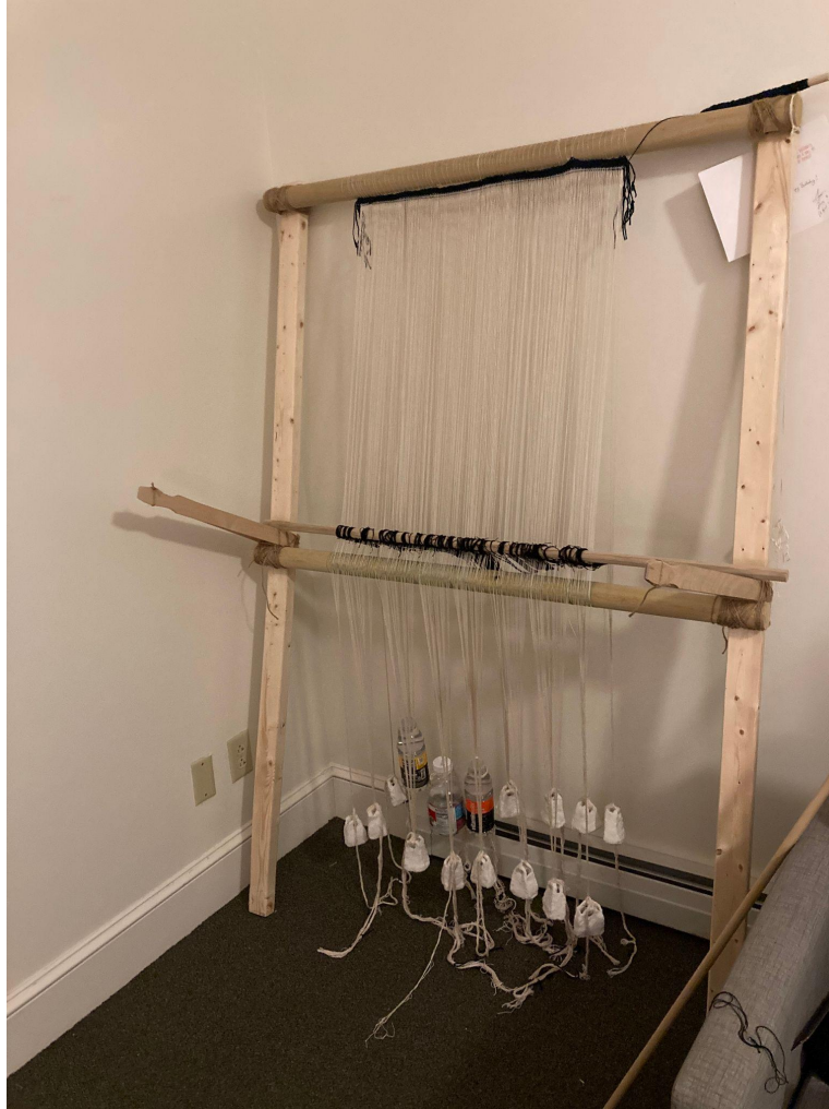
Figure 12: Warp attached to the loom weights 107
