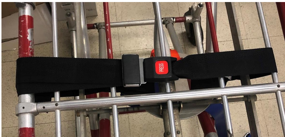
Figure 10. Device-Cot Strap Attached to Ambulance Cot
