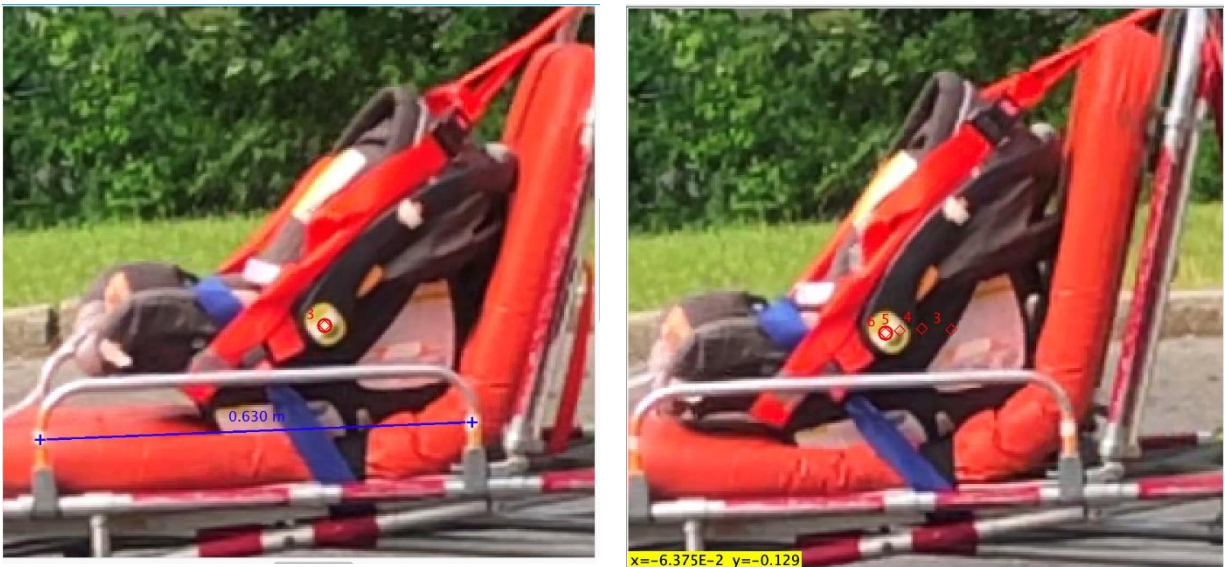
Figure 17: The image on the left demonstrates the initial starting point for the positional video analysis, it also shows the reference scale that was used to create the coordinate system for the analysis. The image on the right demonstrates the point mass analysis that was used to track the movement of the CRS as a result of the stopping force.
