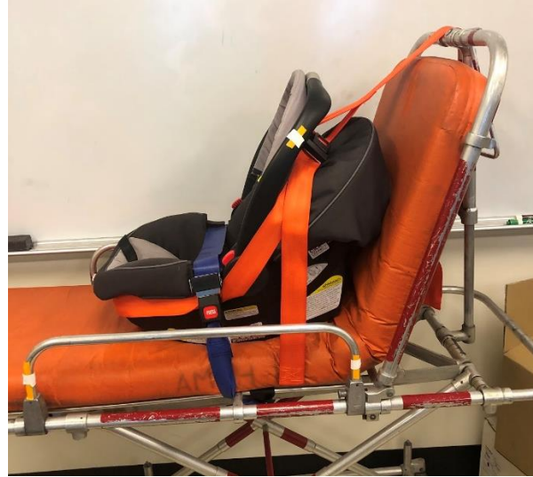
Figure 14. Full Strapping Pattern Assembly
