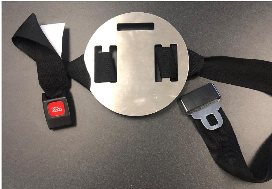
Figure 9. Device-Cot Strap Attached to Aluminum Base
