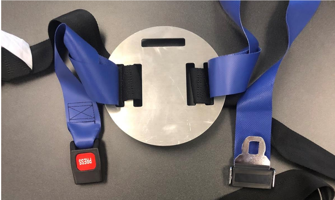
Figure 11. Belt Path Strap Attached to Aluminum Base
