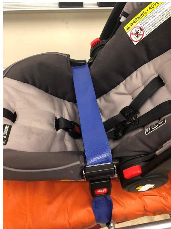
Figure 12. Belt Path Strap Securing RF-CRS to Ambulance Cot
