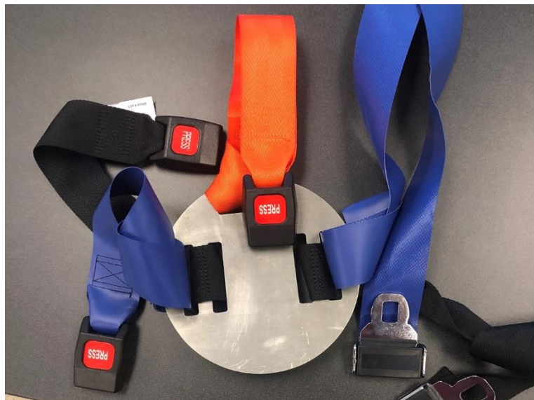
Figure 13. Rear-Loop Strap Attached to Aluminum Base
