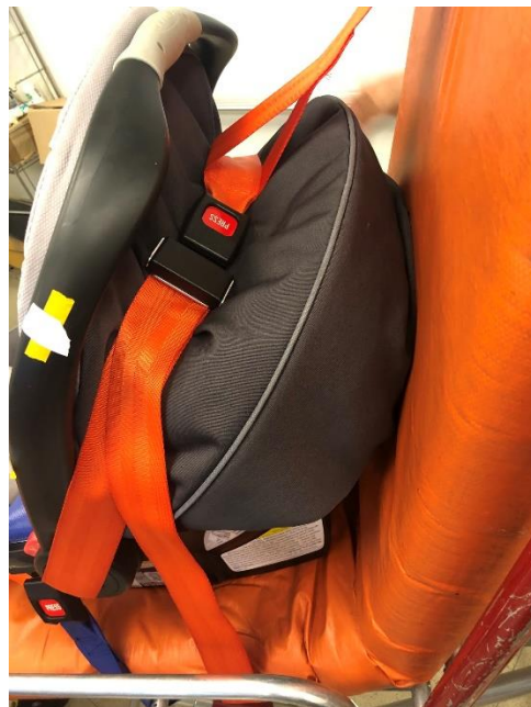
Figure 15. Rear-Loop Strapping Arrangement
