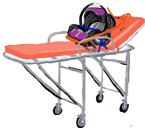
Figure 4. Complete Strapping Pattern of RF-CRS on Cot
