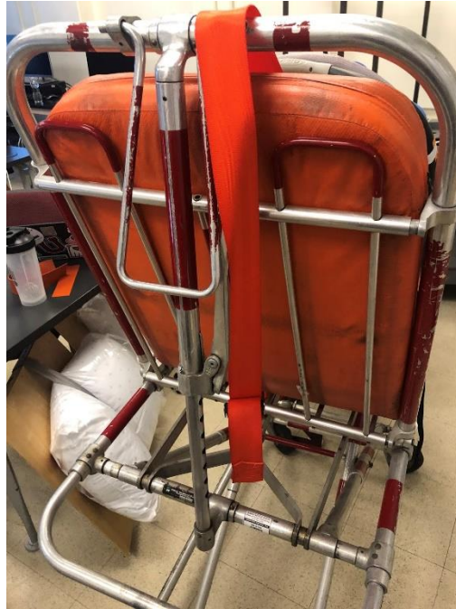
Figure 16. Rear-Loop Path Across Ambulance Cot
