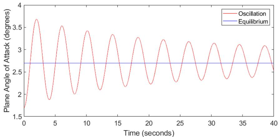
**Figure 10:** This displays a rough phugoid approximation of the Aero 2020 advanced plane displaced one degree from its equilibrium point found earlier,  $2.7^\circ$ , without inputting this information. This confirms the equilibrium angle, and when the tail area is increased the oscillation decays faster, correlating to a higher damping ratio and a more stable craft.
