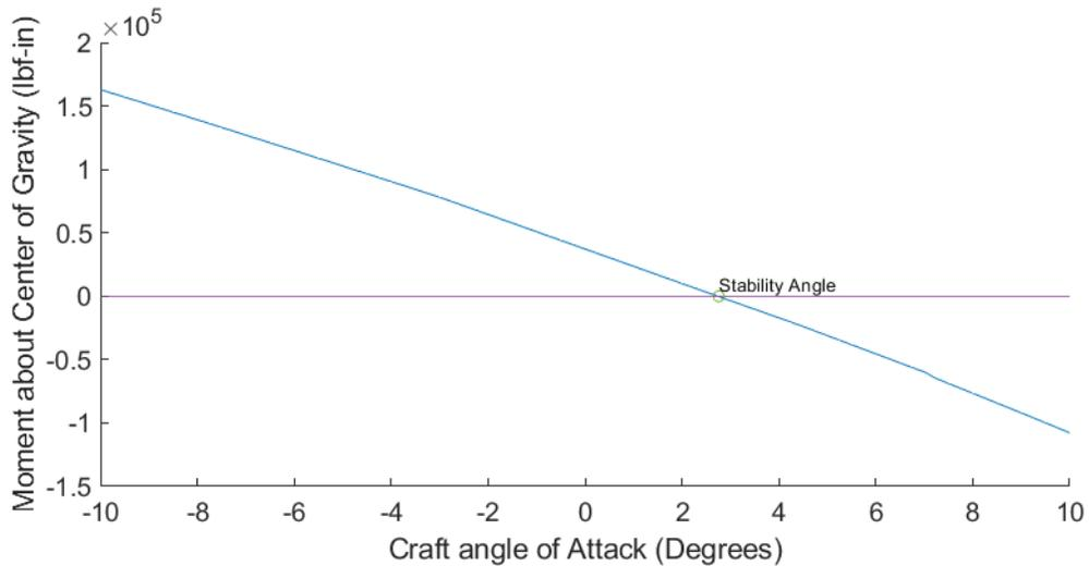
**Figure 9:** Union College 2020 Aero Advanced plane showing at its equilibrium angle (2.7°) it has a negative moment derivative with respect to angle, meeting the conditions of equation 1.
