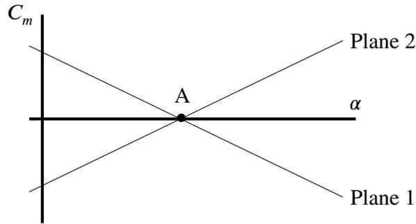
**Figure 4:** Example Moment Plot for Static Stability presenting Moment ( $C_m$ ) vs Angle of Attack ( $\alpha$ ). Point A indicates equilibrium, Plane 1 shows positive static stability (angles above equilibrium express a negative moment pushing it back down to A), and plane 2 shows negative static stability.
