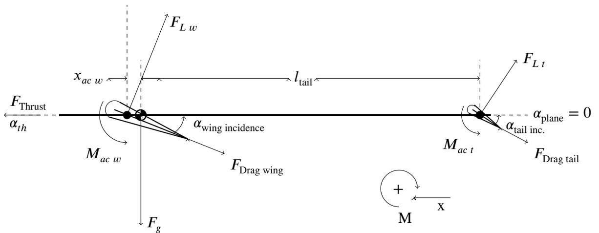
**Figure 6:** Moment Plot for Static Stability presenting at  $\alpha = 0$ , and including the possibility for the wing and tail to have an angle of attack relative to the craft, an angle of incidence. The direction of positive x and positive moment are indicated in the lower right, and variables are explained in the List of Acronyms.
