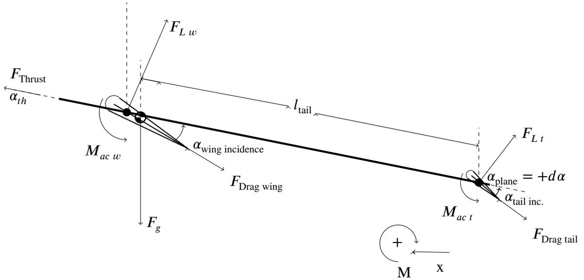
**Figure 7:** Moment plot for static stability presented at  $\alpha = d\alpha$  with all other dimensions the same as figure 6.
