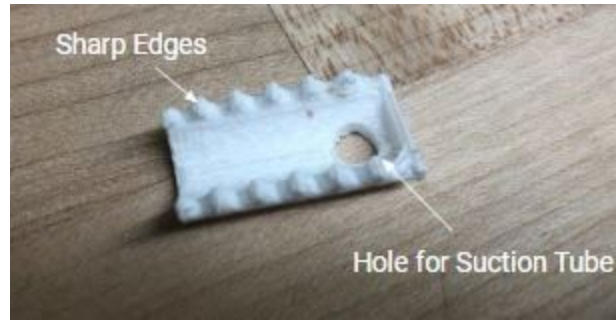
Figure 13: 3D printed tip showing the jaws and the hole where the suction is inserted
