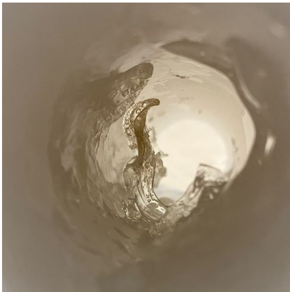
Figure 5. The mucus loaded into the tube for testing.
