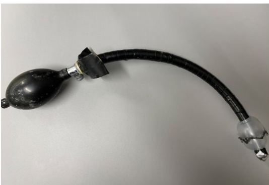
Figure 4. Breathe Easy prototype at a 5:1 scale. Made with a blood pressure pump and endotracheal tube along with the 3D printed ring for the balloon.
