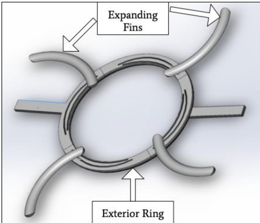
Figure 2. Exterior Ring design with Expanded Fins
