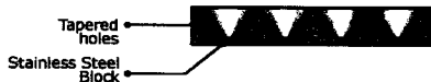
Figure 2-1: A side view of the closed-bottom mold used in the RSCE drying technique. The mold consists of 16 wells arranged in a 4 well by 4 well fashion [1].
