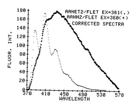
A Comparison of the Fluorescence Spectra of 9-CONEt2  $\qquad \text{and } 9\text{-CONH2 in Water.}$
