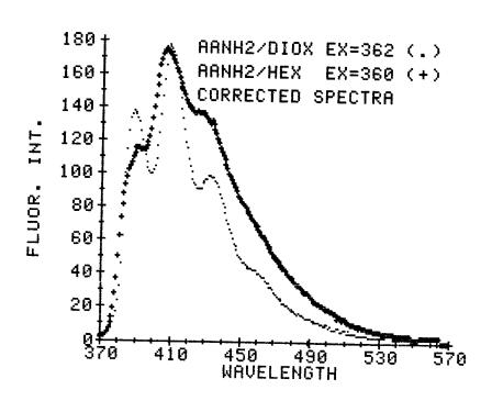
A Comparison of the Fluorescence Spectra of 9-CONH2 in  $\label{eq:Water and Acetonitrile.}$
