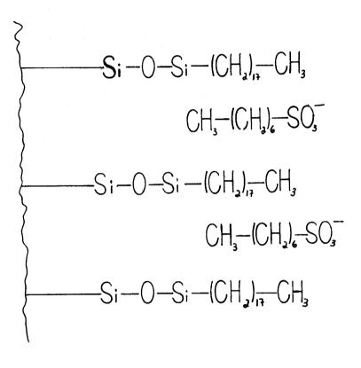
onto the packing surface for any significant length of time, and the acids would therefore be difficult to resolve. With the 1-heptanesulfonic acid to provide a polar site for adsorption, however, the acids are retained and are resolvable. Reservoir B was 100% acetonitrile.
