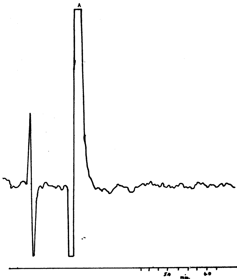
Figure 3. HPLC chromatogram of diethylether. Flow rate: 1.5 ml/min. Detection wavelength: 380 nm. Sensitivity: 005 AU/mV. Peak A: diethylether.
