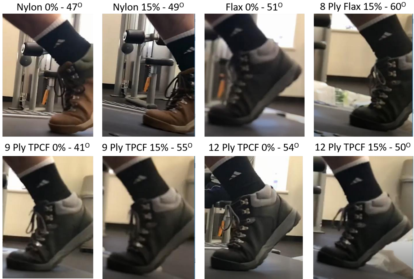
Figure 18: Each material, percent grade of the treadmill, and angle of dorsiflexion are provided. While the nylon test proved to have the boot slightly out of frame during the crucial moment of the boot flexing, an angle measurement was still able to be calculated. It is also important to note the fact that the iPhone 7+ captured a better focus on certain tests over others.
