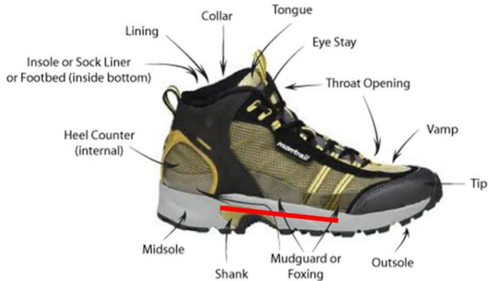
Figure 5: This annotated picture comprehensively shows the components of a hiking boot. The shank (which is hidden in the midsole of the boot) is represented with the red line. The midsole of the boot is responsible for a majority of shock damping when walking or running. The tip of the boot is a durable rubber that is tear and abrasion resistant. The upper of the boot (not labeled) is the main fabric or leather. Within the upper of the shoe is typically a series of waterproofing materials to keep the foot dry.
