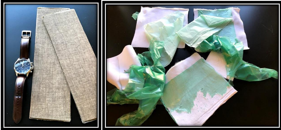
Figure 8: Flax planks with a balsa core were fabricated to illustrate the wastefulness of autoclaving. The waste material (right) includes: bagging material, bleed cloth, flash tape, sealing tape, and non-stick plastic.
