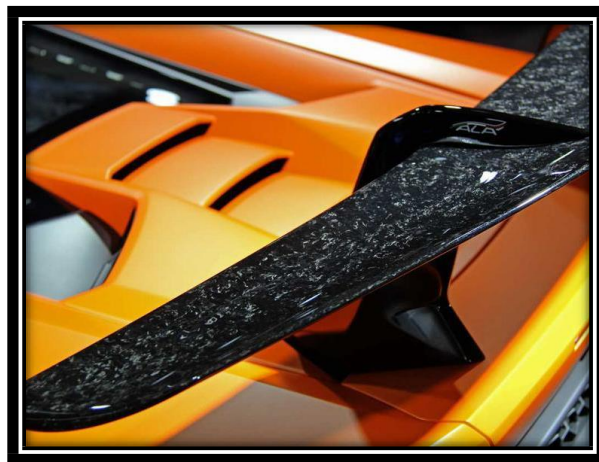
Figure 6: Forged carbon (BMC) is used in the wing of the 2018 Lamborghini Huracan. BMC is used in composite applications where anisotropy is desired. The shiny luster of a BMC composite also provides a unique appearance in the supercar industry [9].
