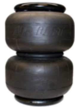
Figure 3a: An example of a traditional double bag suspension system.
