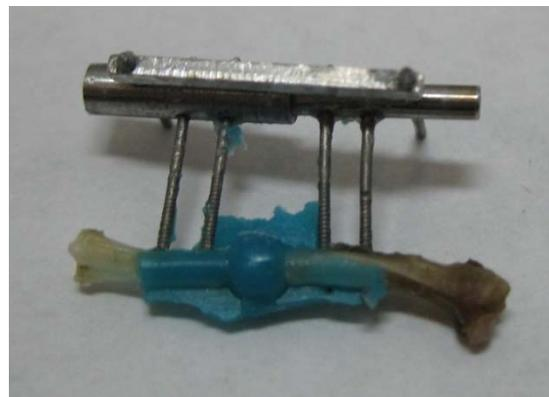
Figure 10: The fixator attached to the tibia with a mock soft callus at the site of the fracture.
