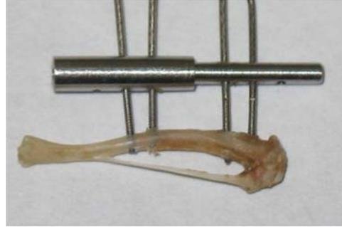
Figure 9: The fixator attached to a tibia.
