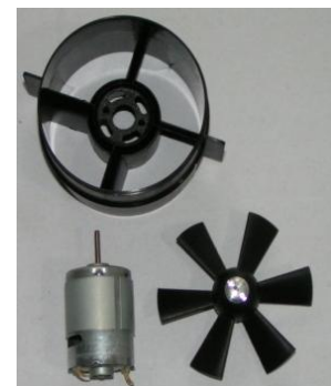
Figure 10: Electric Ducted Fan Assembly
