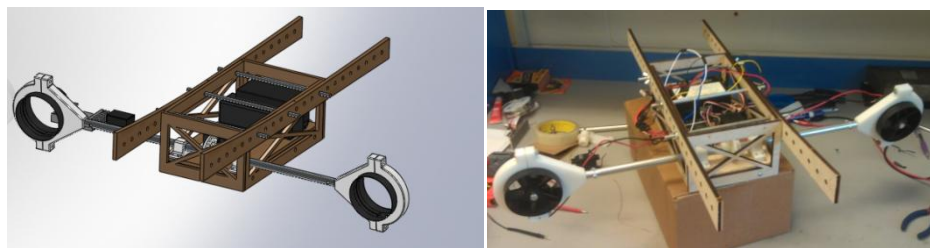
Figure 18: Airship Gondola: CAD Rendering (left), Fabricated Assembly (Right)
