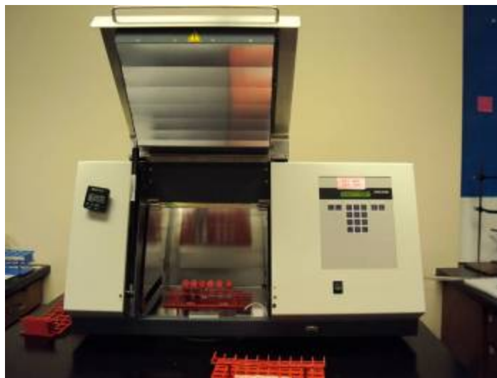
Figure 28. Solar Simulator used in testing photodegradation of methylene blue.
