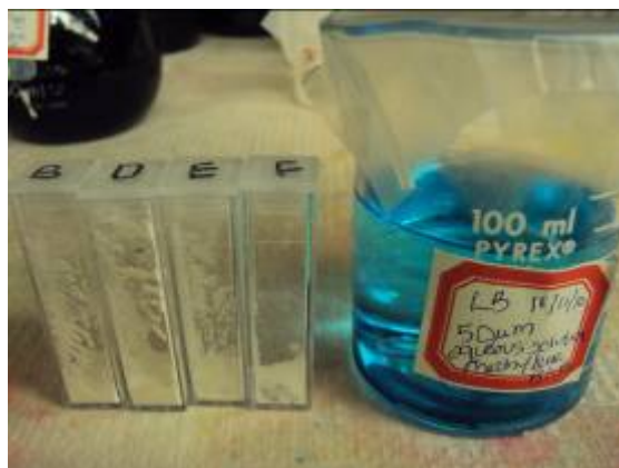
Figure 33. Aqueous methylene blue solution and aerogel samples to add to each test tube.
