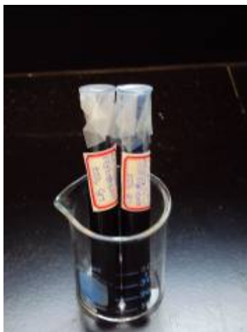
Figure 29. Initial set-up of simple PCO experiment using methylene blue.
