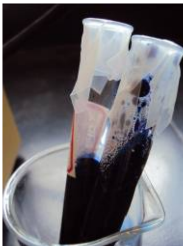
Figure 29. Initial set-up of simple PCO experiment using methylene blue.
