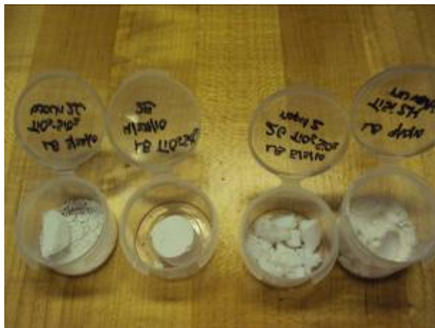
Figure 4. Titania-silica monoliths fabricated using the Rapid Supercritical Extraction method.
