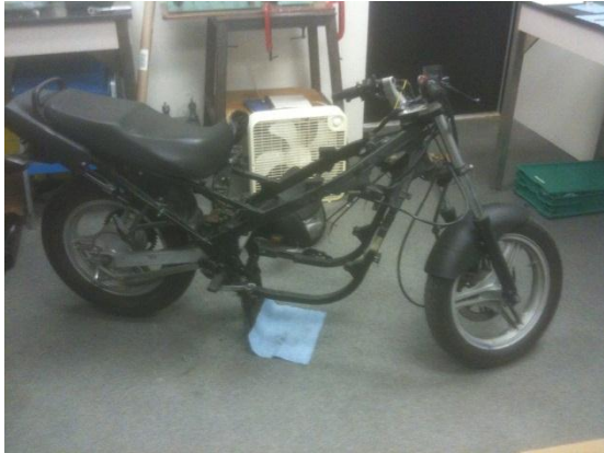
Figure 21: Motorcycle chassis with IC engine & drive train removed
