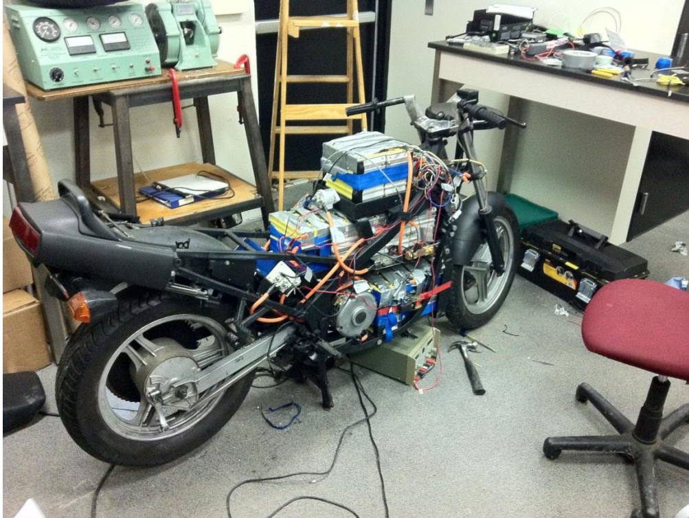
Figure 23: Completed drive system mounted to project bike
