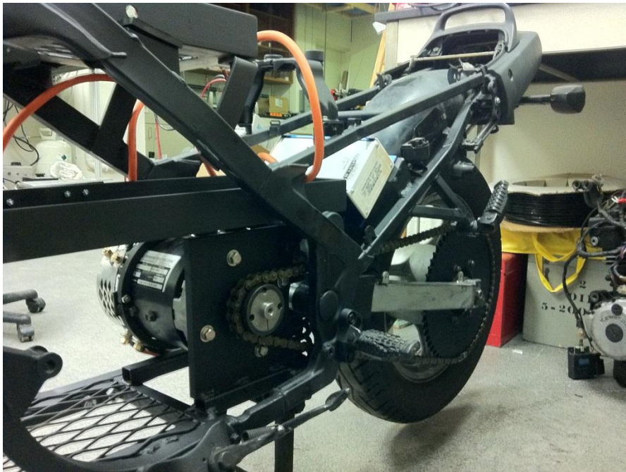
Figure 19: Chain and sprocket drive train final configuration
