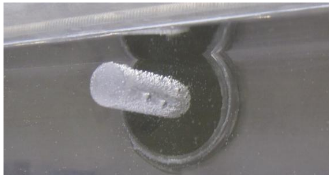
Figure 5.8: Submerged coated test piece in cross flow
