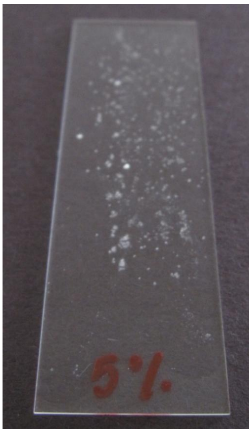
Figure G.1: 5% aerogel by weight to Nafion; 30 minute powder
