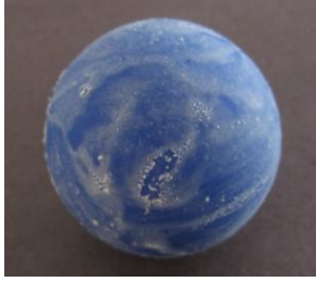
Figure M.2: Aerogel surface coating on practice rubber golf ball
