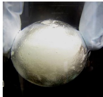
Figure 3.4: Coated ping pong ball submerged in water
