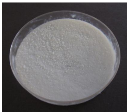
Figure C.4: Aerogel powder crushed for 20 minutes with a mortar and pestle using propanol as a solvent
