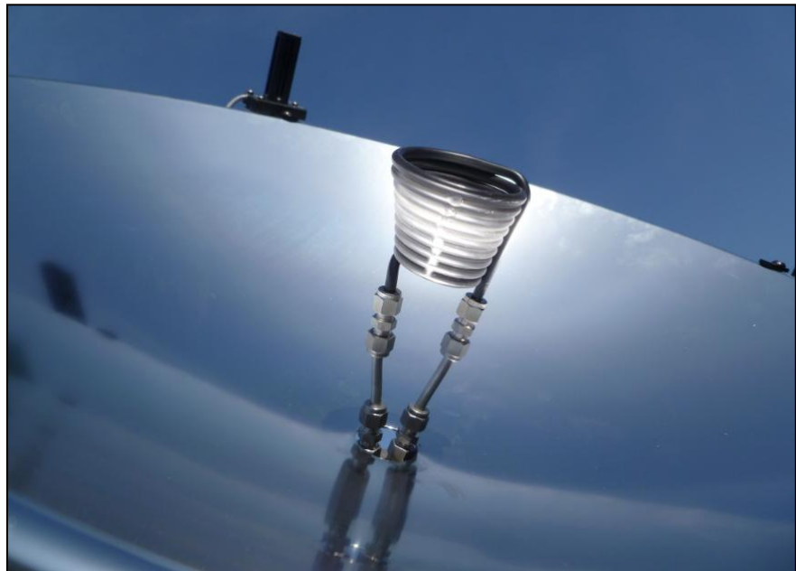
Figure 16: Solar Thermal Receiver in the Focal Point of the Dish
