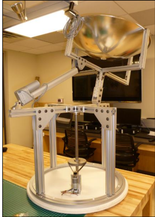
Figure 8: Completely Assembled Tracking Structure
