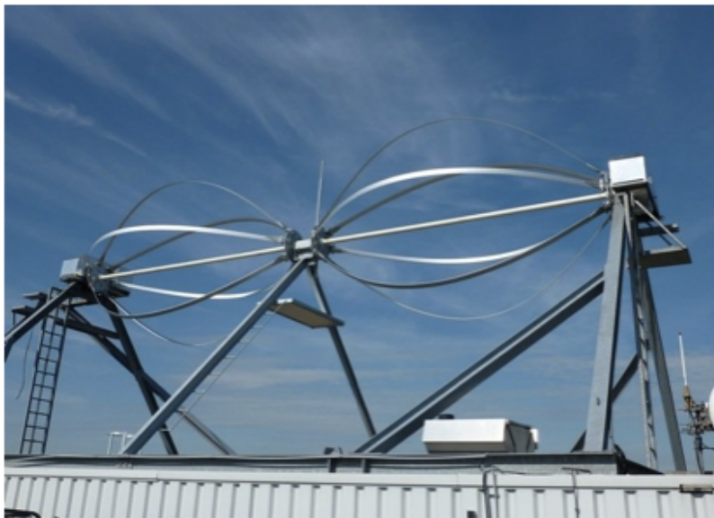
Figure 2: A picture of a windwall turbine, which is a horizontal axis wind turbine, with the axis in a fixed position so wind is caught in one direction.
