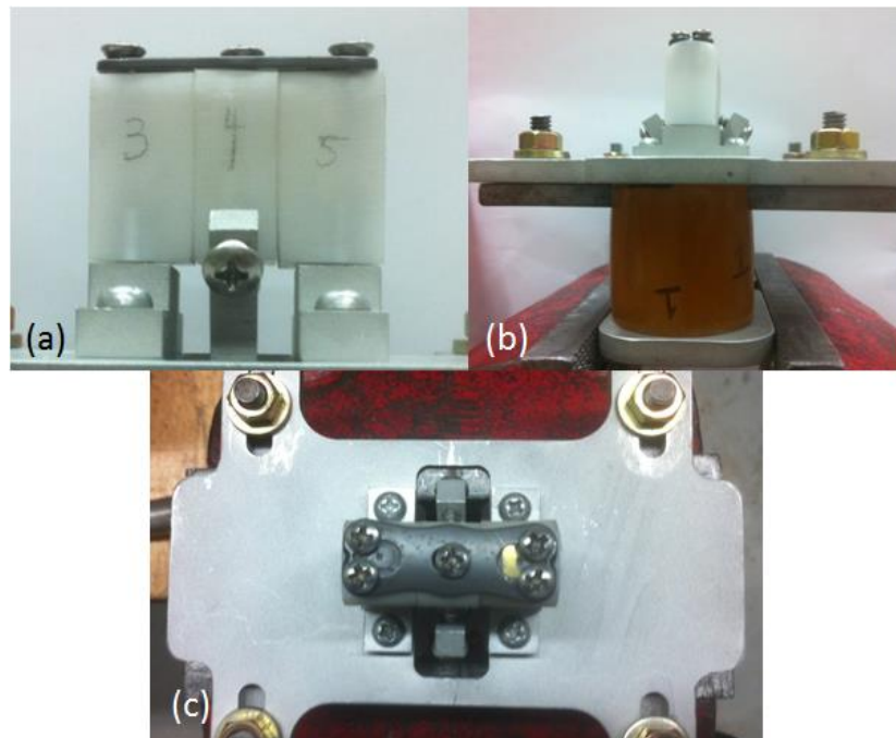
Fig. 36: Post-Test Pictures for Anterior Standard Three Point Bending Test – Part (a) shows a side view of the fixture with the numbers referring to the cervical vertebra they represent, part (b) shows a front view looking from superior to inferior, while part (c) shows a top view of the fixture with implant in place.
