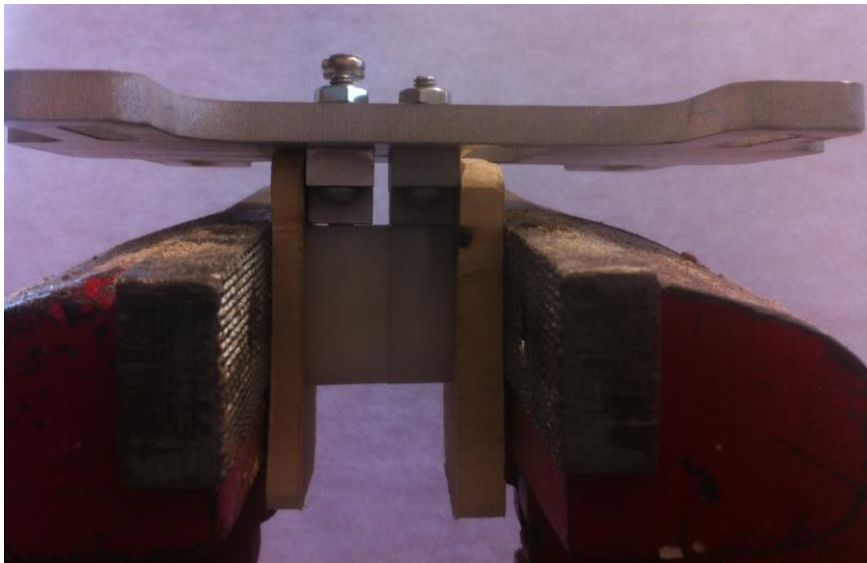
Fig. 30: Fastening of Delrin to Front Plate – For the anterior terminal three point bending fixture, after the first Delrin vertebra has been fastened to the front plate, the second one can more easily be secured. After positioning the left unfastened vertebra correctly, it is wedged between two slits of wood and tightened in a vice. The proper orientation will then be maintained during fastening.
