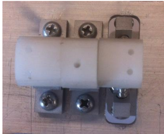
Fig. 33: Pre-Drilled Implant Holes – The alignment of the pre-drilled holes where the screws will be fastened to secure the implant are shown.
