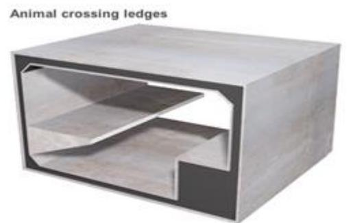
Figure 6. Example of European “ecoculverts” with built in ledge.
