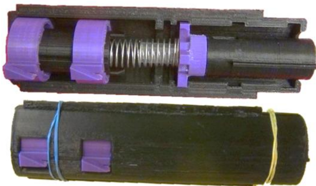
Figure 42: Final Prototype Assembled. Shown here as both a cross section and held together with rubber bands.
