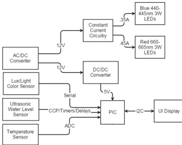
Figure 5. Electronic Block Diagram
