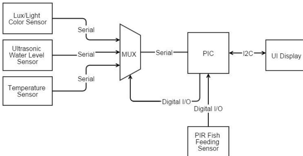
Figure 1.Originally Proposed Electronic System Block Diagram
