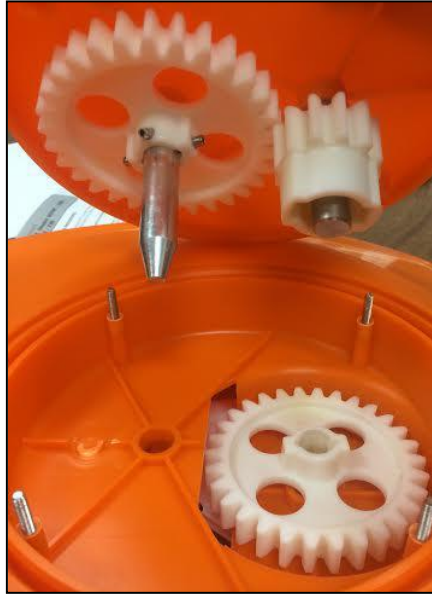
Figure 10 – Salad Spinner with built in gear train.
