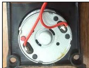
Figure 36 – AC generator in hand crank flashlight
