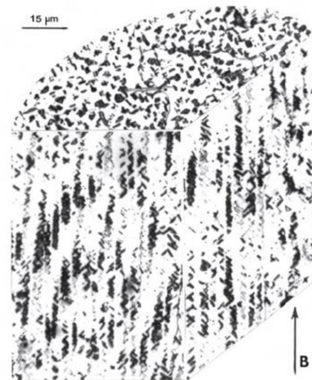
Figure 3: A light optical microscopy image of the grain structure of an Inconel 625 made cylinder made via electron beam melting. The highly oriented columnar microstructure runs parallel to the build direction shown by arrow "B". Figure from [3] Murr, L., Martinez, E., Amato, K., Gaytan, S., Hernandez, J., Ramirez, D., Shindo, P., Medina, F., and Wicker, R., 2012, "Fabrication of Metal and Alloy Components by Additive Manufacturing: Examples of 3D Material Science," Journal of Materials Research and Technology, 1(1), pp. 42-54.
