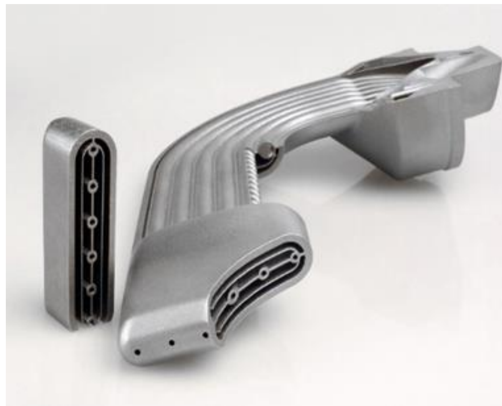
Figure 1: A gas emissions rake developed using AM. Fine internal geometries make the part light weight. The small tubes inside of the part allow gas to flow through the monolithic part. Figure from [1] Richter, T. 2015, "Metal Additive Manufacturing: Component Design for Successful Commercial Production," Metal AM, 1 (1), pp. 37-45.
