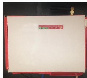
Figure 28 - Implementation of user notification LEDs
