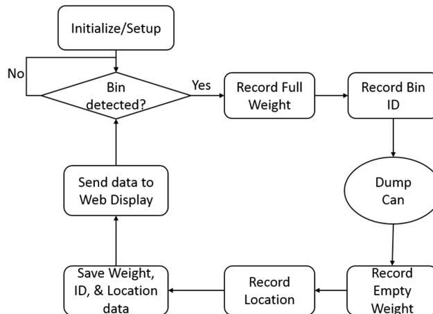
**Figure 14 - Overall procedural flow diagram**
