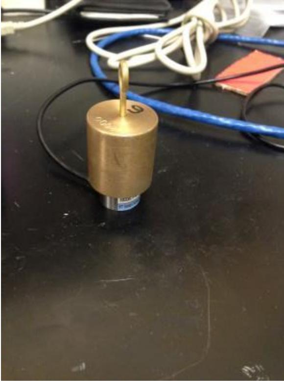
Figure 20 - Load cell testing with 200g weight
