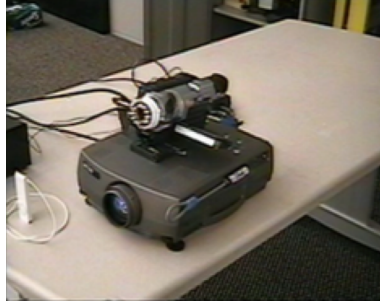
Figure 2: Truong et. al.'s device. Sitting on top of the projector is the Sony HandyCam used for sensing, and the projector is used for blinding cameras in the area of the device. [10]
