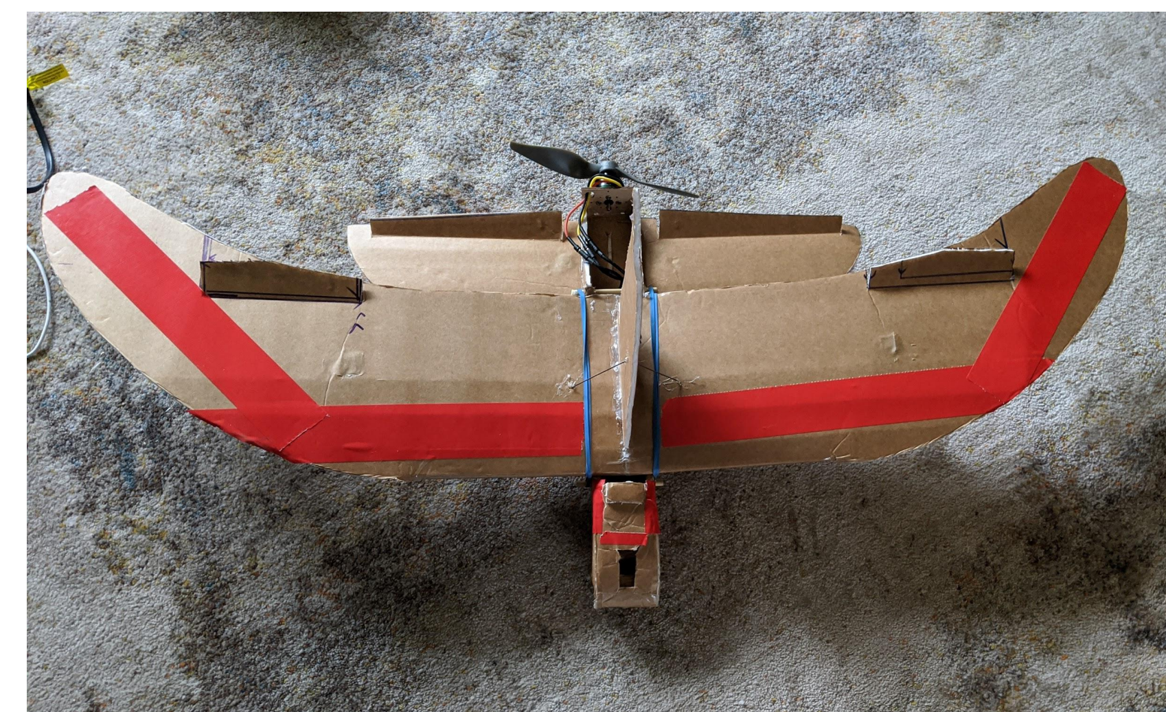
Figure 4: Modified flight test system with expanded wings, modified tail, ports and slots in fuselage for electronics organization, and standard control surfaces.
