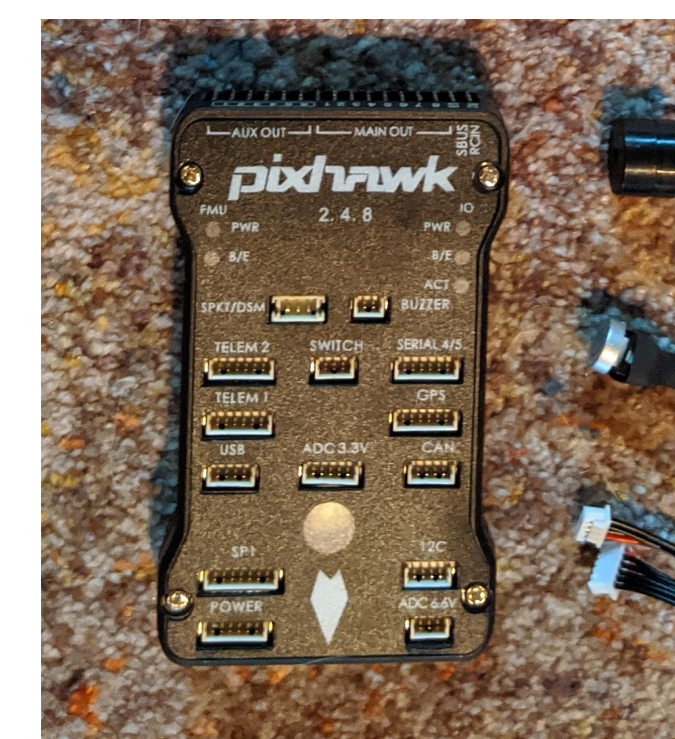
Figure 6: A pixhawk PX4 flight controller. Data collection system for analog pitot tube readings, gyro sensor, and accelerometer readings.
