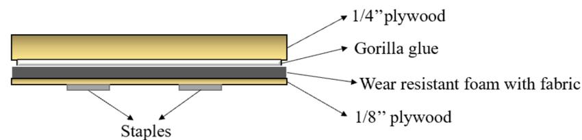
Figure 3. Schematic of the Composite Material
