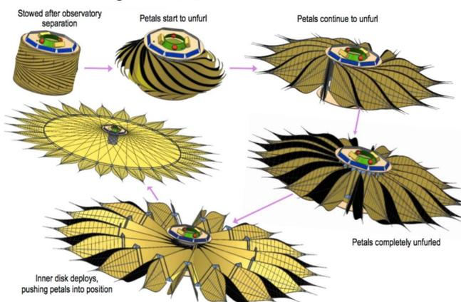
Figure 1. The Deployment Process of *Starshade* [3].
