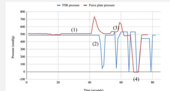
Testing protocol performed on Pasco Force Plate (red) and FSR (blue). Both show comparable pressure at heel when subject is vertically resting, and significant changes in force during periods of turning and repositioning.
