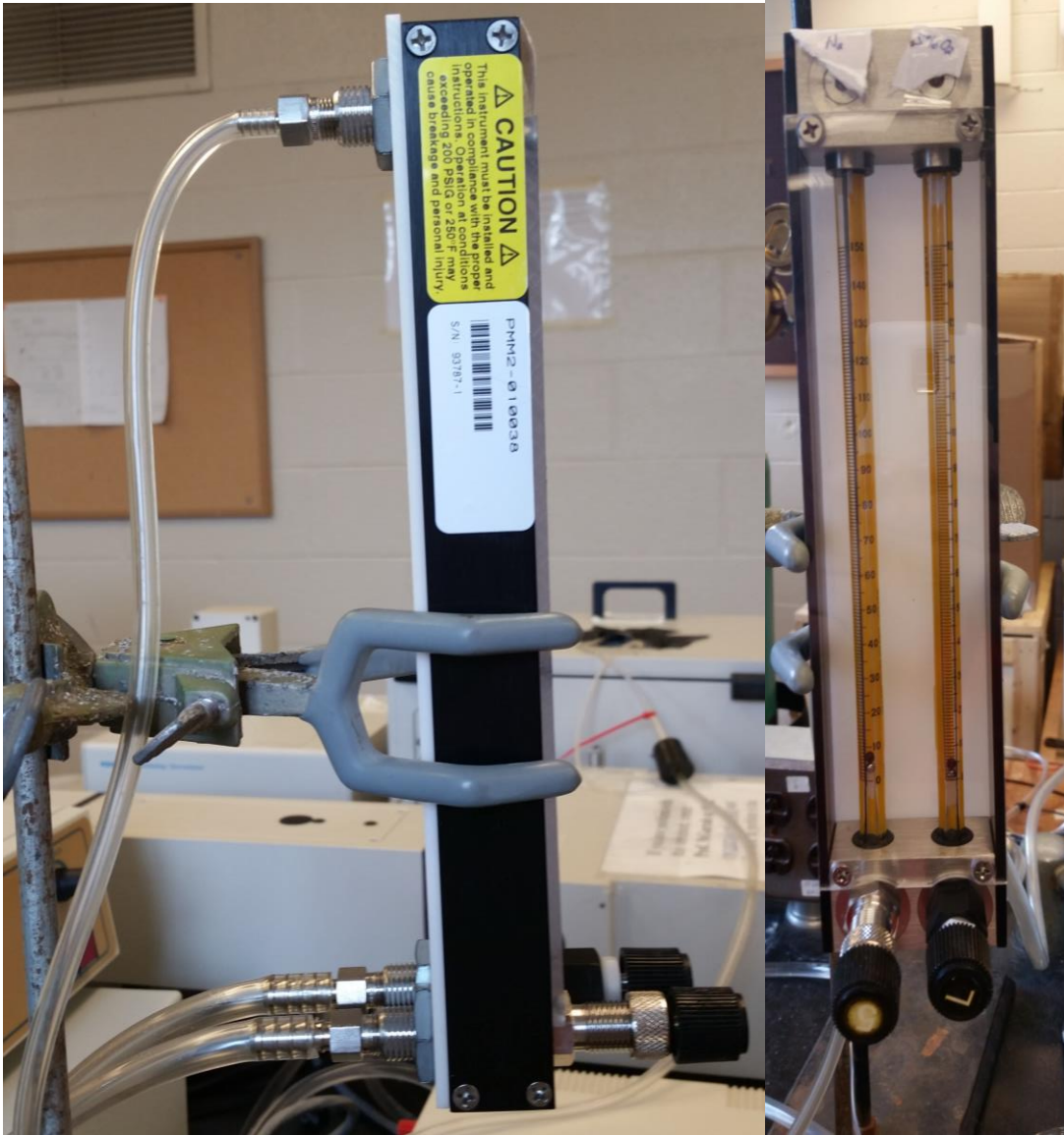
Figure 11: Left- Front of gas proportioner. The left knob controls the flow rate of N_2 , while the right knob controls the flow rate of the gas blend being used. Right- Side view of gas proportioner. The two tubes at the base are the inlet tubes from the N_2 and gas blend tank. The tube at the top is the outlet tube for the proportioned gas.
