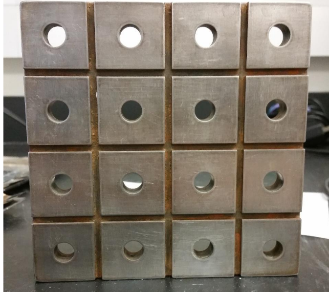
Figure 7: 125 x 125 x 12.5 mm mold, with 16 wells, each 9 mm wide.
