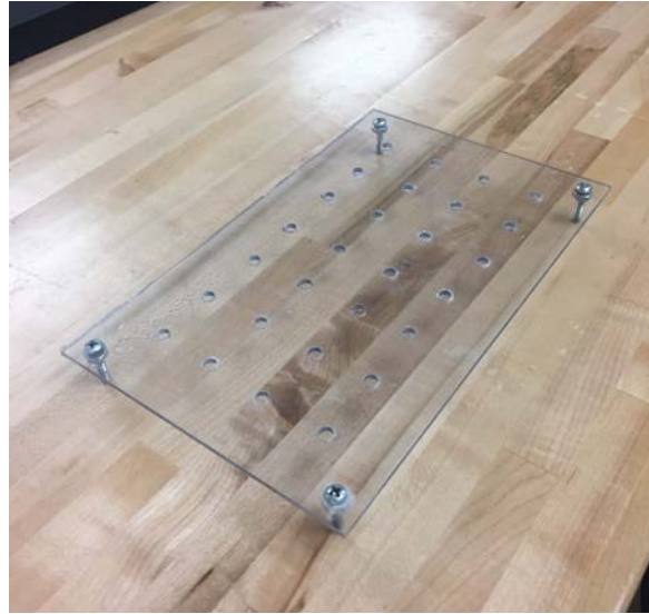
Fig.15. Plastic grate used in experimental modeling of ITES storage container.
