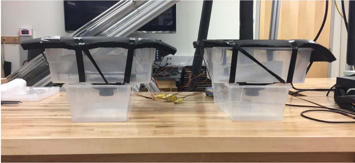
Fig.14. Experimental setup used for the large ice storage container test with the metal grate. The storage container on the left contains the metal grate with the ice block on top of it while the storage container on the right has the ice block on the bottom of the container.
