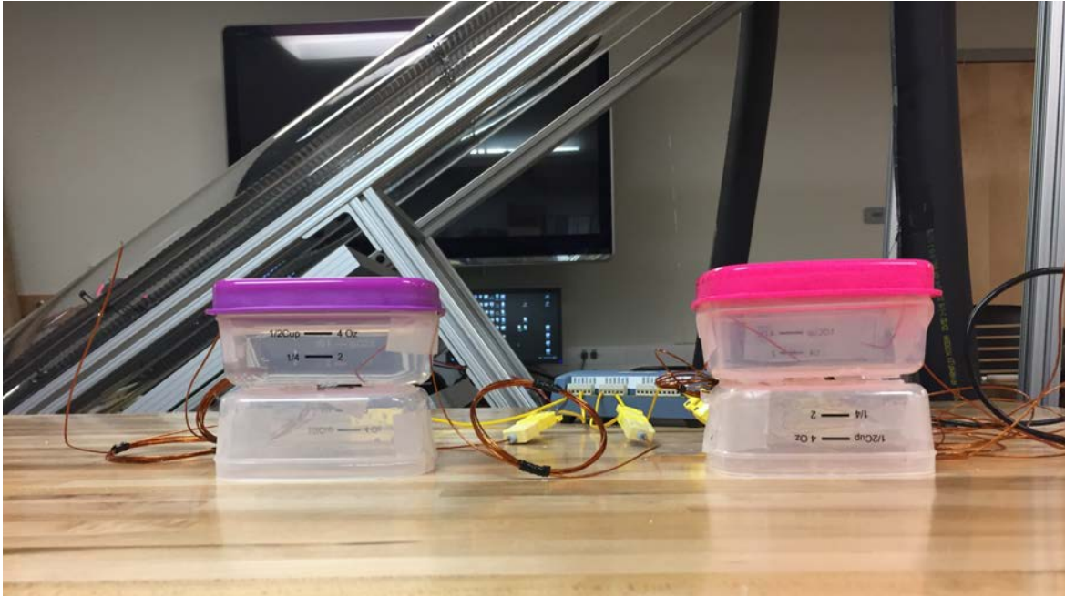
Fig.11. Experimental setup of the two ice storage tanks. The tank with the purple lid was used as the original tank model with no drain and the tank with the pink lid was used as the new tank model with the drain.
