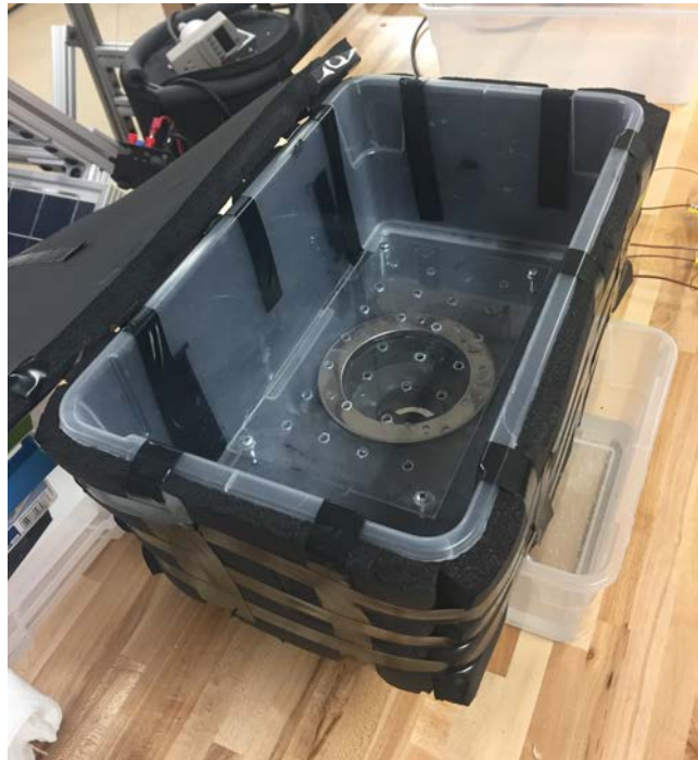
Fig.17. Final ITES storage container with a drain, a plastic base grate, and 1 inch thick insulation around the sides, top, and bottom of the container.
