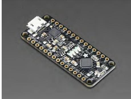
**Figure 7: Chosen Microcontroller for Prototype- Adafruit Metro Mini**
