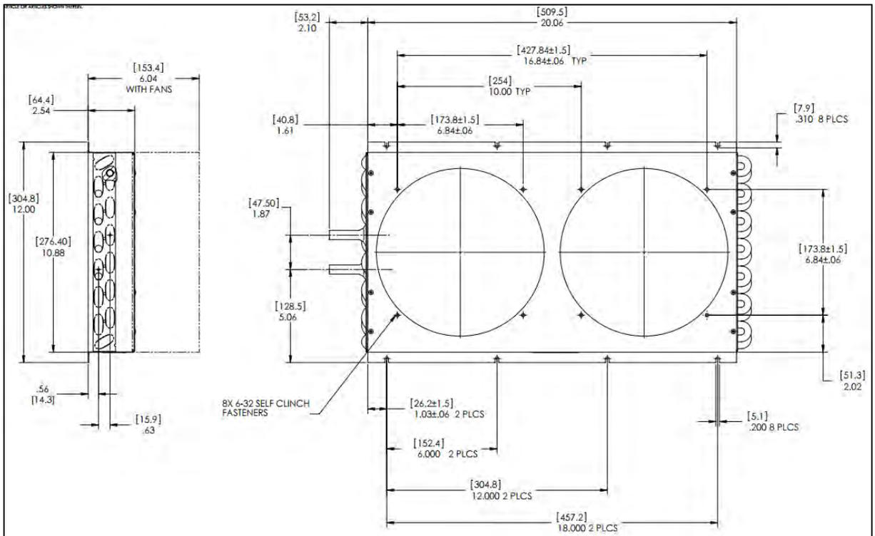
Figure 5: Detailed drawing of heat exchanger [11]
