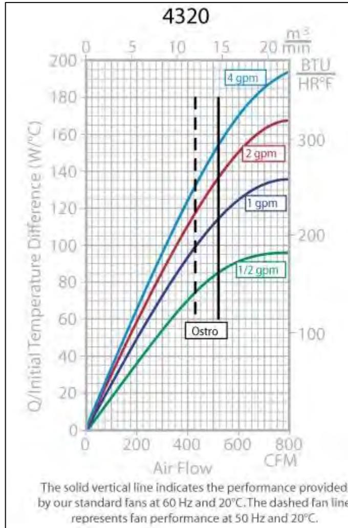
Figure 6: Performance Curve of Heat Exchanger [11]
