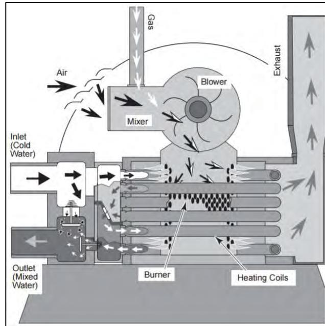
Figure 1: Gas pool heater diagram [7]
