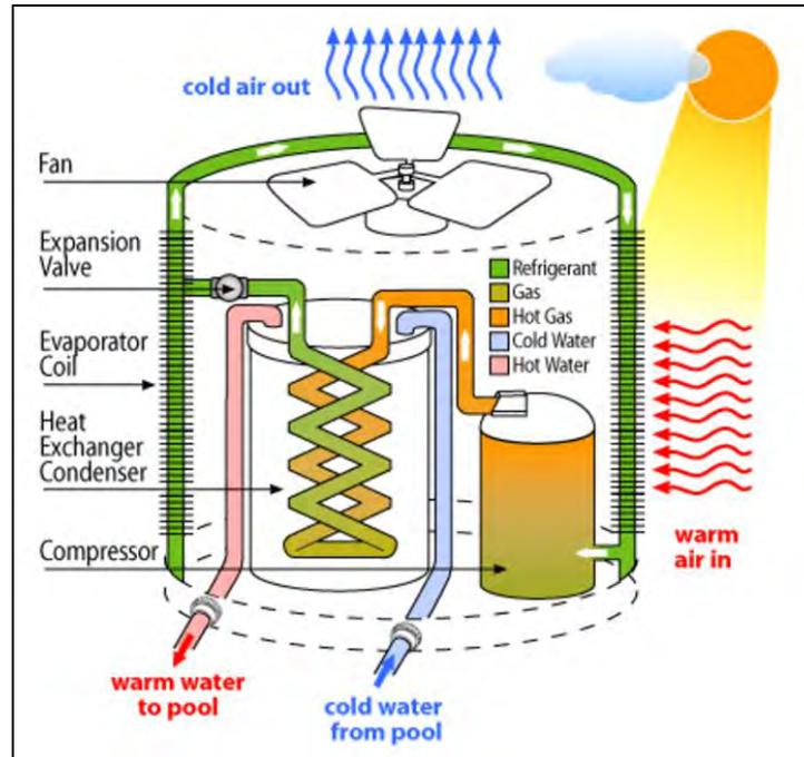
Figure 2: Heat pump pool heater diagram [8]
