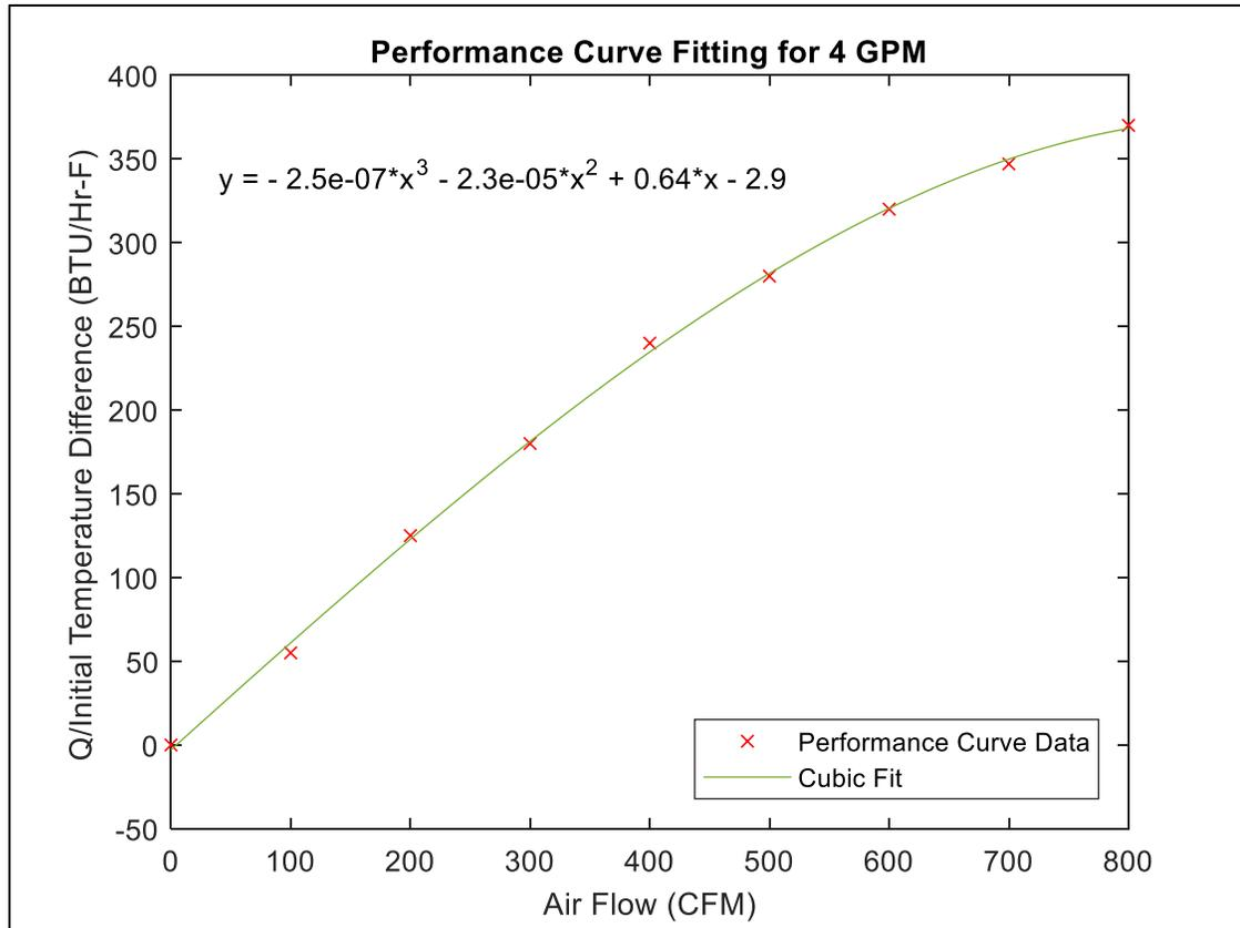
Figure 7: Performance Curve for 4 GPM from MATLAB
