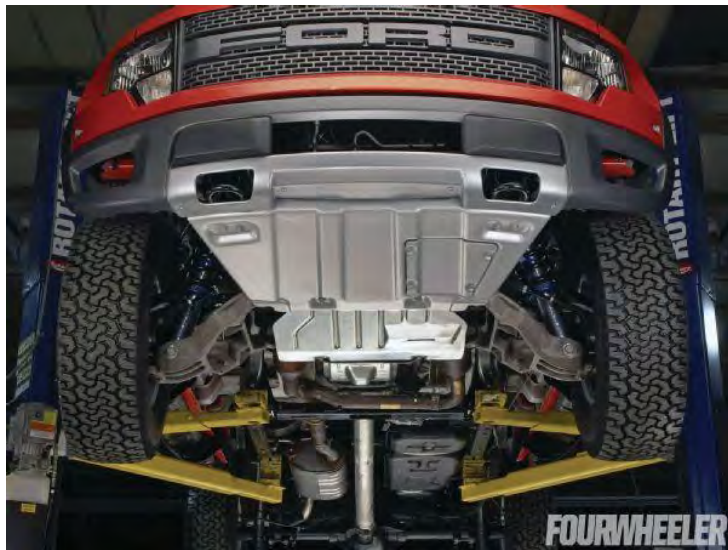
Figure 3 - Independent front suspension on the 2017 Ford Raptor (Frontend Fued - IFS Vs. Solid Axle., 2013)
