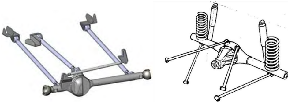
Figure 4 - Three link front (left) and four link rear (right)
