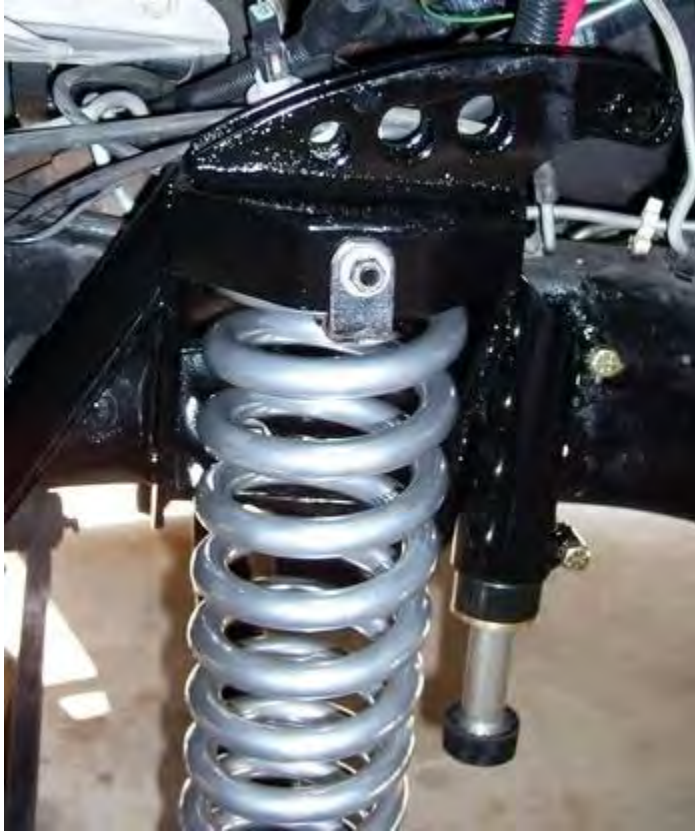
Figure 13 – Hydraulic bump stops (Ansell, Suspension Link Construction)
