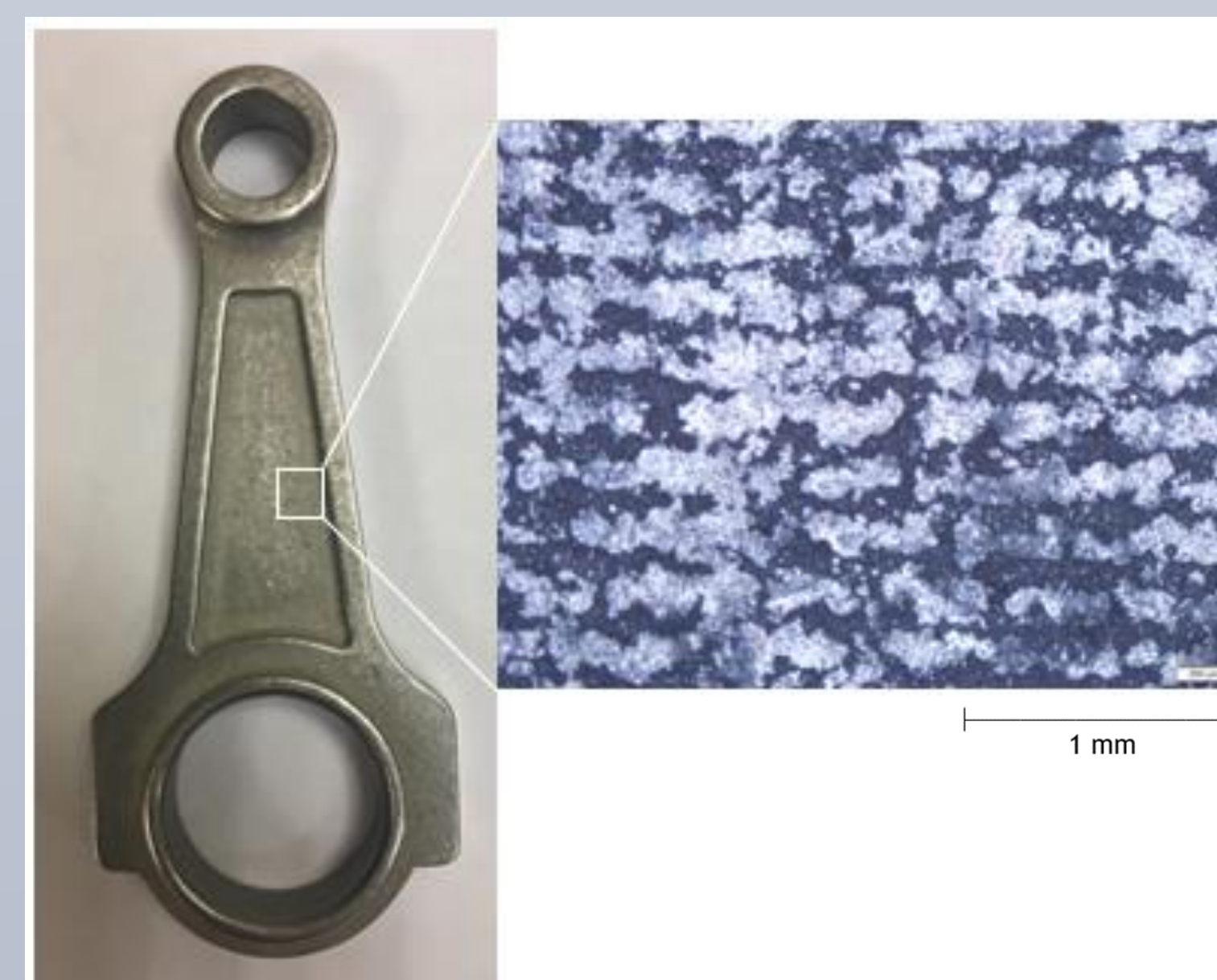
Figure 5: Image of part printed with DMLS process and 50x magnification view.
