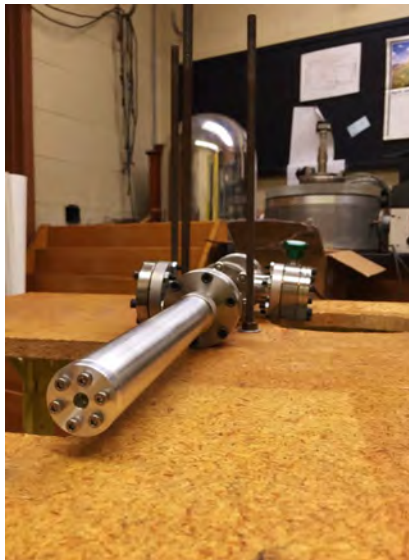
FIGURE 2.5: A photograph of the external beam pipe showing the opening and the Kapton foil window. In this photograph, the beam pipe is not attached to the scattering chamber of the accelerator.
