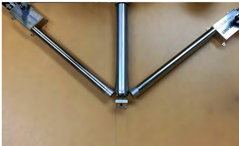
FIGURE 2.6: A photograph of the setup of our external beam facility. The detectors, an SDD x-ray detector on the right in the image and a CdTe \gamma -ray detector on the left, come in at 45 degree angles to the external beam pipe in the center. The samples were attached to the small metal rectangle located in front of the external beam.
