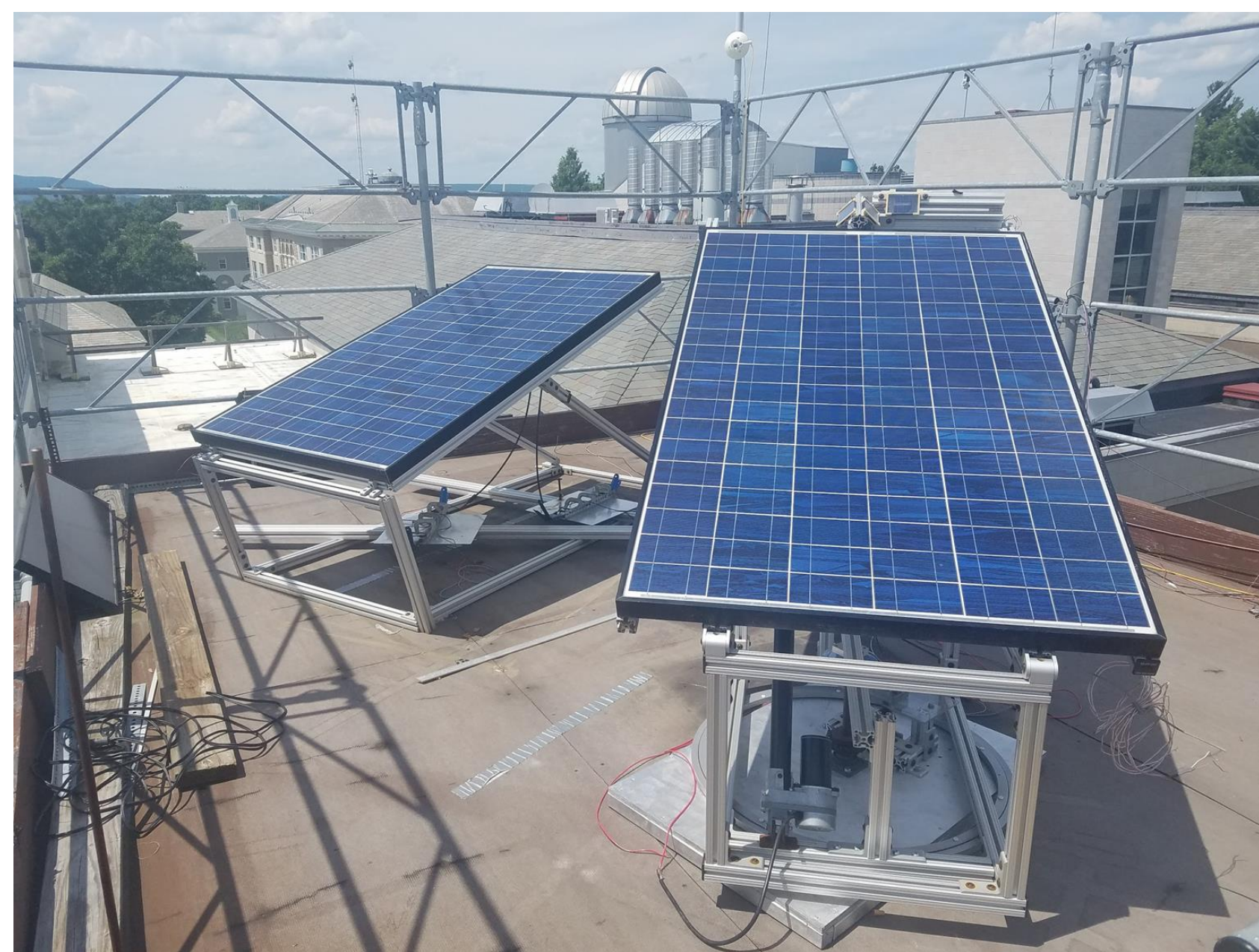
Figure 1 . Stationary panel alongside tracking panel.
