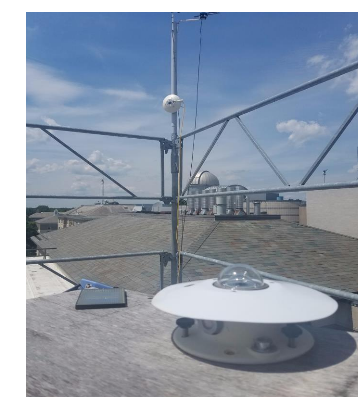
Figure 4. Vertical and horizontal pyranometers.
